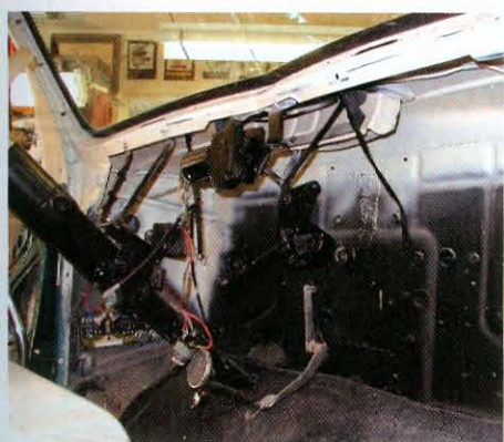
5) Here's the firewall after complete removal of the original insulator. We painted the light color to facilitate photography. The original mounting holes along the top will be reused to mount the new insulator. Note all the pressed-in reinforcements. These eliminate the need for the vibration-killing sound-insulation strips.
