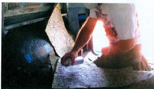
24) Next comes a very important step: spraying a matching, even coat of adhesive on the insulation piece. We're sure you've noticed that the insulation sheets are installed foil side in. This allows the rag side to absorb the heat and the foil side to block it from getting into the interior.
