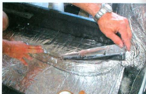
27) After all the insulation is glued in place, it's time to seal every joint and seam with the supplied foil tape. This forms a one-piece inner skin of insulation with no small cracks or holes to allow heat to penetrate.
