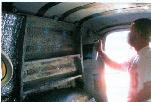
23) With all the pieces cut to fit each position, Cox begins the sidewall installation. Here, he's using the supplied spray can to apply an even coat of adhesive to the area. Note the fume-filtering facemask.
